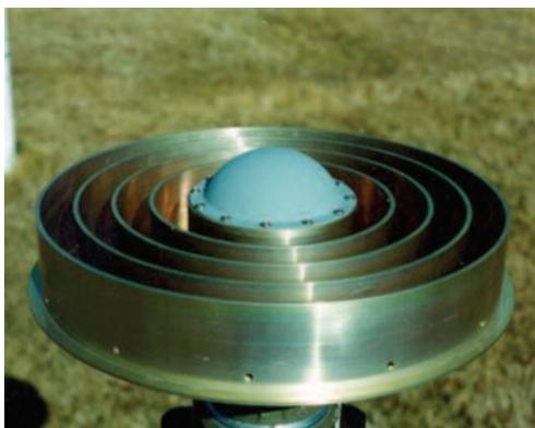
Figura 2 Antena Choke Ring
